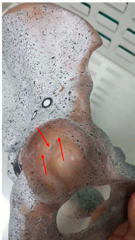
Fig. 12. The form of failure under ultimate load; the arrow indicates the location of the crack.
